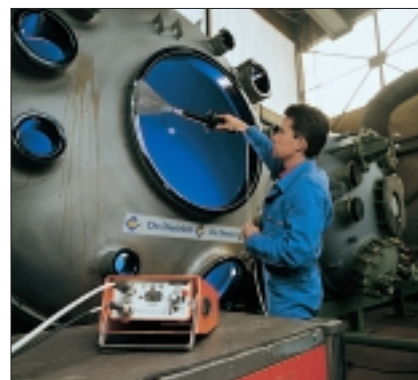
POROSCOPE® HV20 to test for pores and pinholes in nonconductive coatings.
