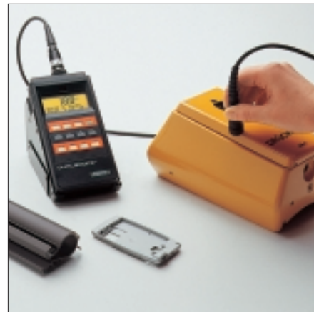
Measurement of the paint coating thickness on a curved surface using ETD3.3 probe and DUALSCOPE® MP40.
